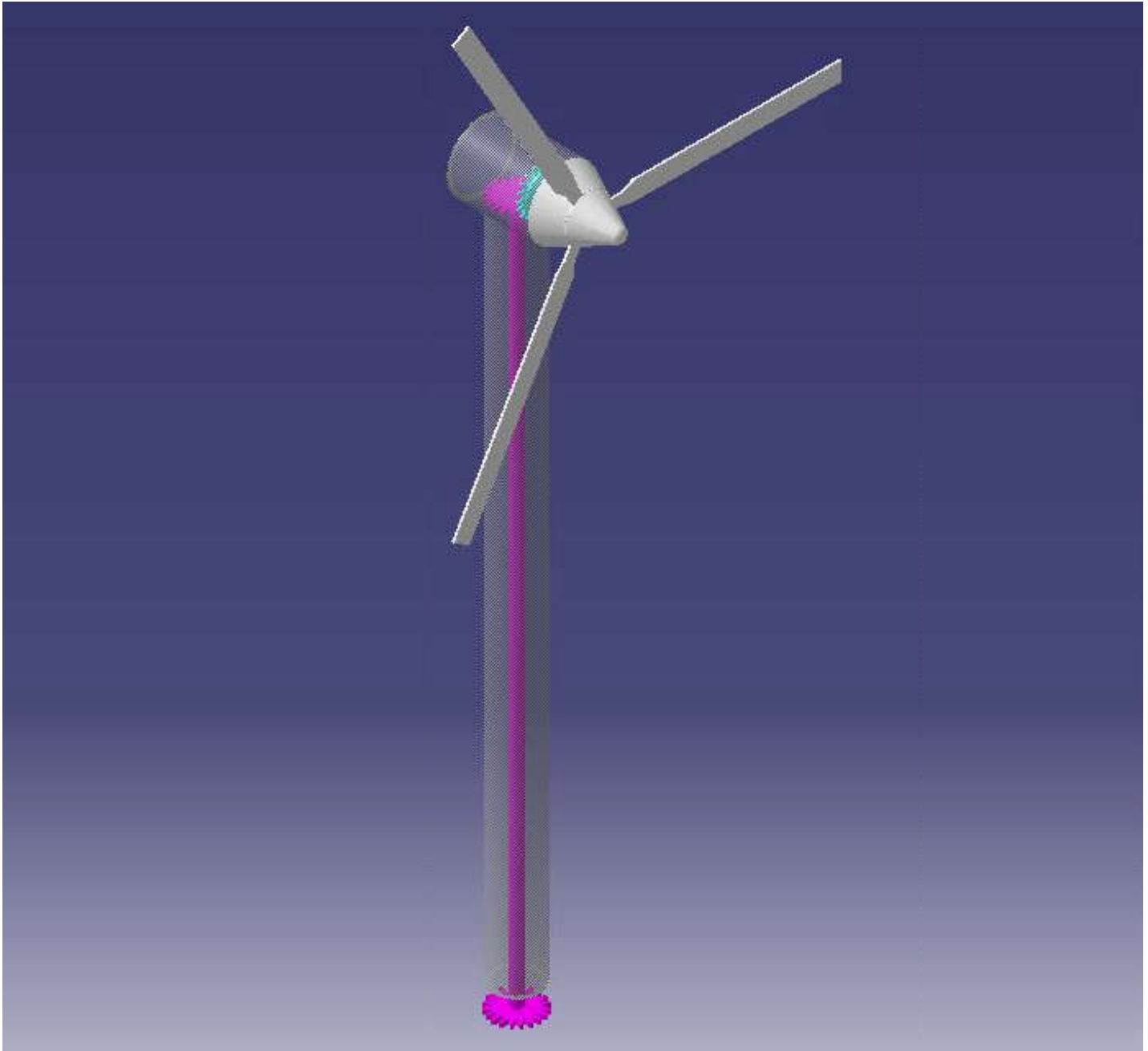
Figure 9 – the new single wind turbine design
