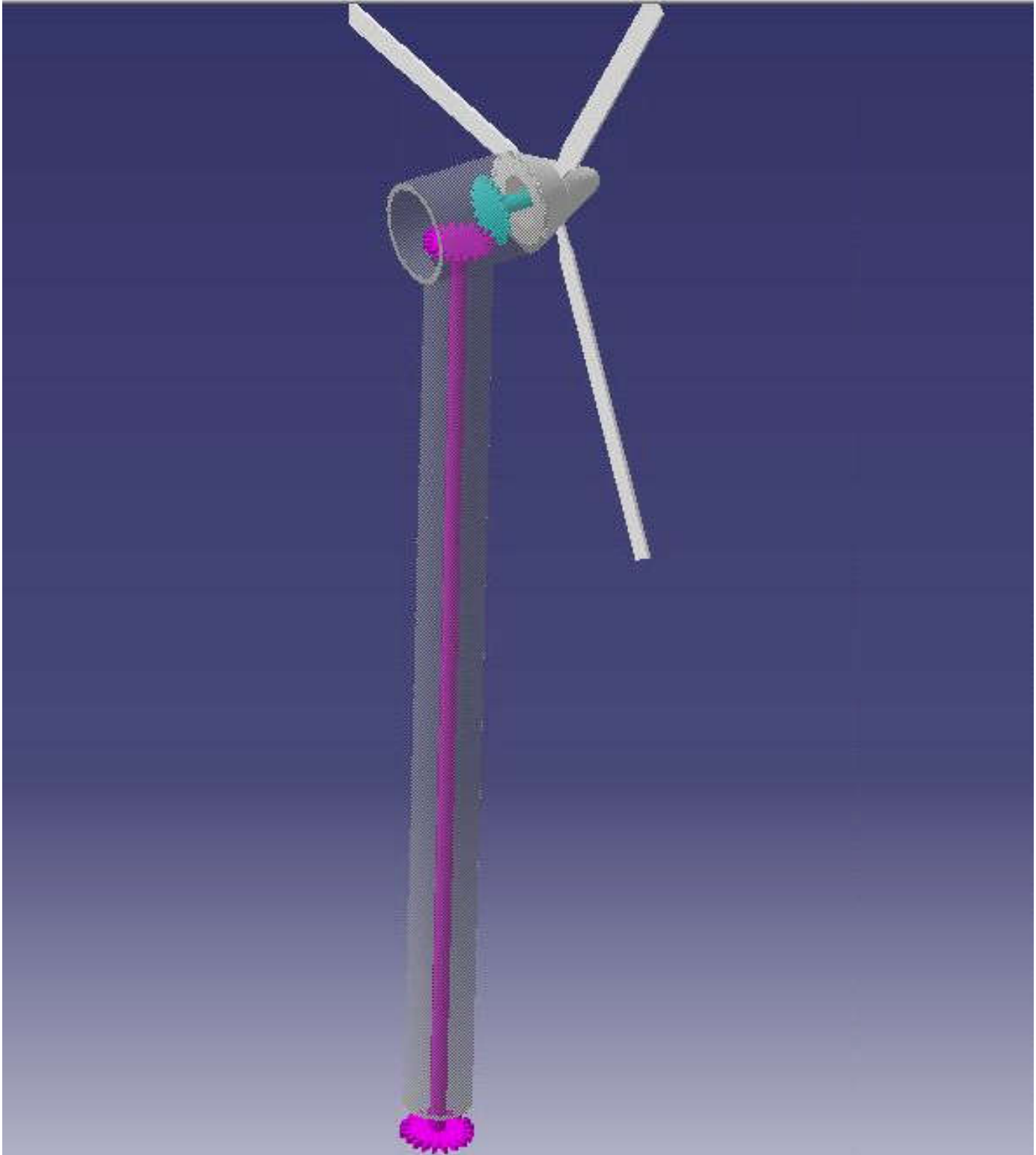
Figure 10 – the new single wind turbine design
